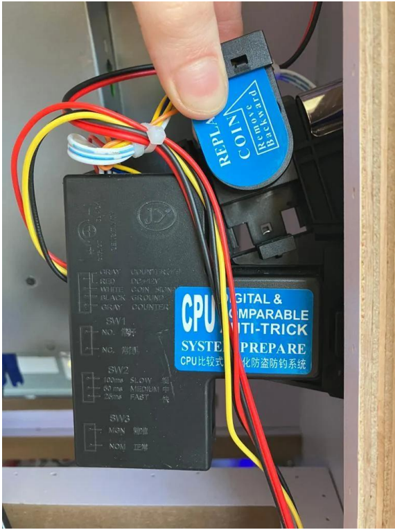
Hold the clamp slide up and place a coin in the slot.
