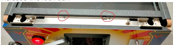
Remove the side profiles.
