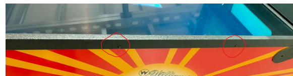
Slide the (heavy) glass plate out.
