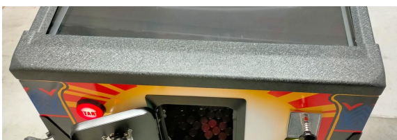
Release the lock bar.
